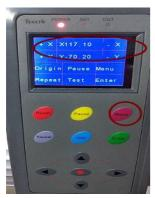
Step 5. Click "Cut" on your computer and the red laser will goes to the second Mark, press your computer keyboard direction button to move the red laser to cover the middle of
