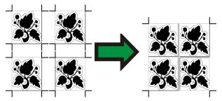
Using a single set of registration marks for multiple jobs allows the jobs to be cut in less time, because the cutter has to process far fewer registration marks. It also saves material that would otherwise be taken up by the extra registration marks. However, it sacrifices some precision in cutting, because the cutting head does not get realigned for each copy.
