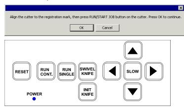
Use the front panel controls on the cutter to position the head of the cutting device over the Gerber registration mark.
