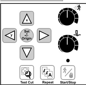
3. Align the sensor light over the first mark (the lower right mark), press the **Set Origin** button on the cutter, and then click **OK** in the software.
