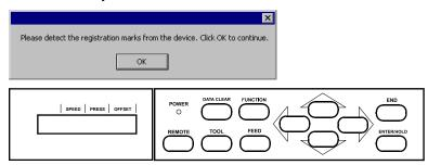
7. Align the cutting head over the first automatic registration mark (lower right if not marked) using the controls on the front panel of the cutter.
