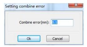
The software automatically merge curves in the selected curves, when these curves merge tolerance is less than the setting of combine error.
