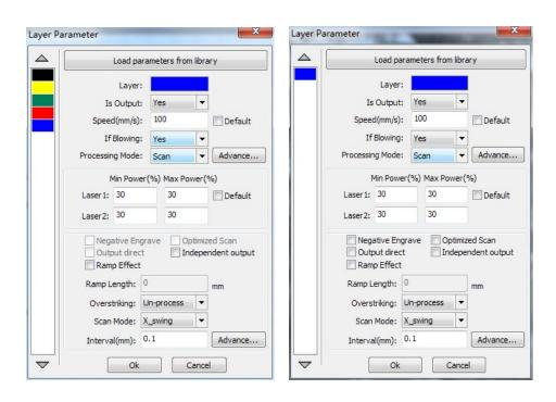
On the left of the dialog box for vector scanning parameters Settings, on the right side of the dialog box for bitmap scanning parameters Settings.
