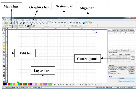
**Menu Bar:** The main function of this software are available through the implementation of the Menu Bar. Execute the menu command is the most basic mode of operation. Menu Bar including: Document, Edit, Draw, Setting, Processing, View and Help.
