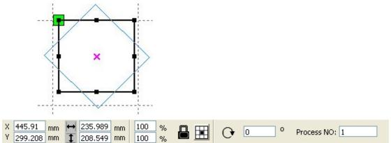
Or directly enter the rotation angle in the Object Properties toolbar.
