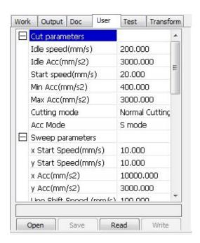
Reading the board parameters must before operating the user parameters.
