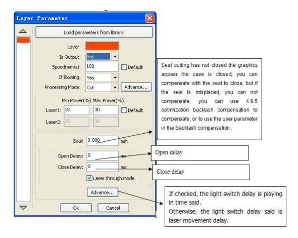
Using the slit width compensation can compensate for the offset between the graphics and the actual output graphics that caused by laser cutting.
