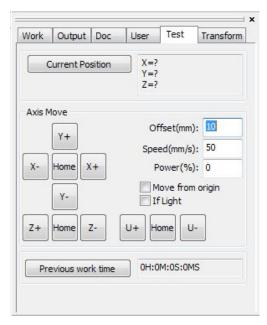
Axis control, can only control one axis each time. You can set the information for axis move, including move length speed laser on-off and laser power.
