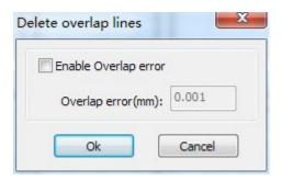
Under normal circumstances do not select the "Enable Overlap error". Removing the overlapping lines when two lines are compared to a good degree of coincidence. If you need to delete overlapping lines, you should select "Enable Overlap error", and set overlap error. Generally do not overlap error set too large, so as to avoid accidental deletion.
