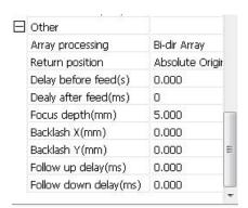
Array processing: Can choose a two-way array and one-way walk array. Two-way walk array: namely array according to the order of cutting back and forth; One-way walk array: always from one direction to another direction to array of cutting. When choose unidirectional arrays, each array element action pattern of exactly the same, fluid movements completely consistent, but better than two-way array is somewhat time consuming. The default choice two-way array
