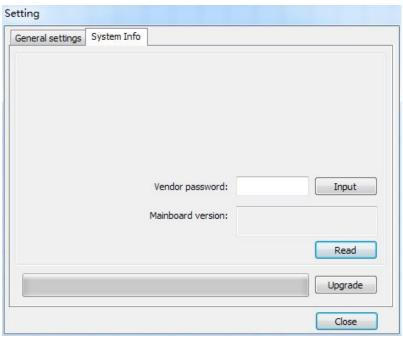
Information on the operation of the motherboard manufacturers need to enter password to view parameters.
