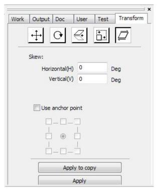
Object can be tilted by the tilting transformation tools. It can be set the tilt anchor and the tilt angle.
