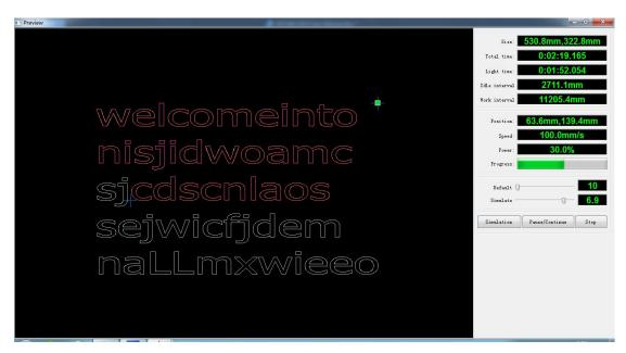
Software supports the preview of the documents to be processed, and you can get some basic information through the preview. For example, the path of the actual output of the processing, general processing time, processing the distance. The machining process can be simulated.
