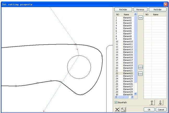
Select the graphics that should be changed the cutting point, it will show all the nodes in the current graphics. Select the starting point, double-click the mouse, it will change the starting point 确定 of the current graphics. After the completion of all changes, click the result of the
