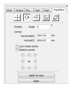
Or use the spin rotation transformation tools to transform. In the rotations transformation tool can be set to the center of rotation and locking center of rotation.
