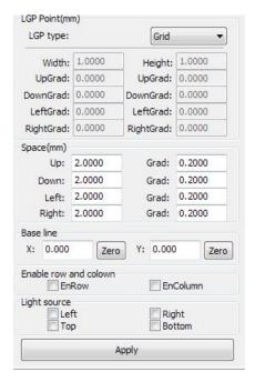
Network is divided into six ways: horizontal, vertical line, elliptical, rectangle, reticle and the grid. Baseline related with light source, the user can adjust the baseline position according to time light source. In the figure above red graticule marker is the baseline, users can move the mouse to baseline, press the mouse, and then drag the baseline to want to position.
