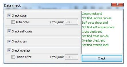
Data check, integration of the closed inspection, the inspection, the inspection, the intersection of the fellowship data overlap a check. The user can select a check, inspection to the problem after data, will be in the dialog box right tip have been found and, at the same time, the problem in selected state graphics. Check-> ruled out repeatedly error-> inspection process until all the data are conform to the requirements of the processing.
