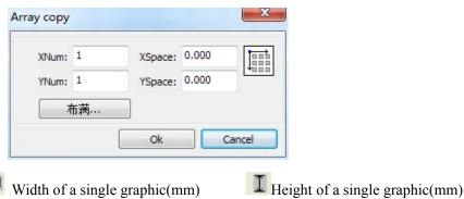
You can array replication object along different directions. The direction of copy is based on the original graphics. Such as choose the array direction lower right, then the original graphic will appear on the upper left corner. wheres if it is to the upper left array, then the original graph appears in the lower right.
