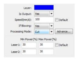
Laser:Software to distinguish between different layers of the graphics processing technology parameters. For scanning processing methods, more are in the same layer bitmaps, and whole as a picture output, if hope each bitmap single output, it can be a graph respectively placed in different layer can.
