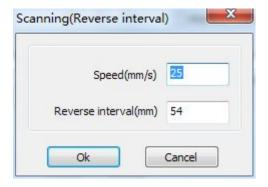
In the interface can modify the current speed of the corresponding backlash.
