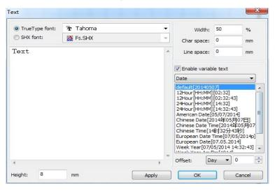
Variable is the date when the current every time processing take the current system of computer time output. Software offers a variety of date format for customers to choose.
