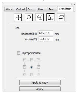
Or use the size transformation toolbar to change the size of object. Can modify the size, choose whether to lock the aspect ratio, and set the position relative to the object to transform.
