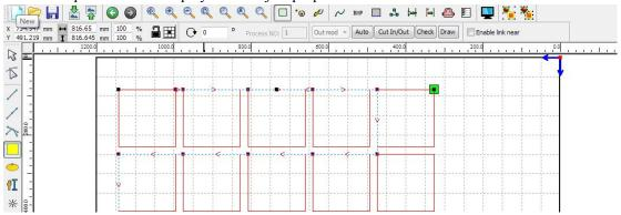
Enter the serial number directly in the processing number, then press the keyboard "Enter" key, or click the plot area, the cutting order will be changed.
