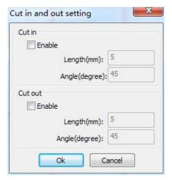
To make cut in/cut out lines, first of all need to enable the cut-in/cut out function.
