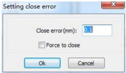
Close error: When distance from the starting point to ending point less than close tolerance, automatic closing of the curve.
