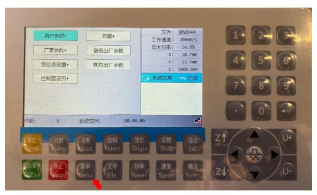
Press "Down" button to select the Controller Setup (+ means has sub-menu)
