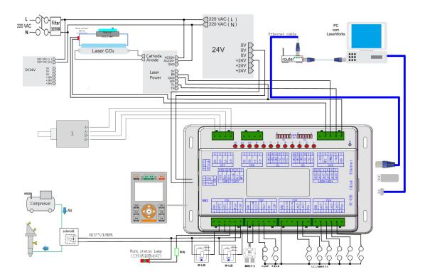
2-1 Electrical connection diagram of control system
