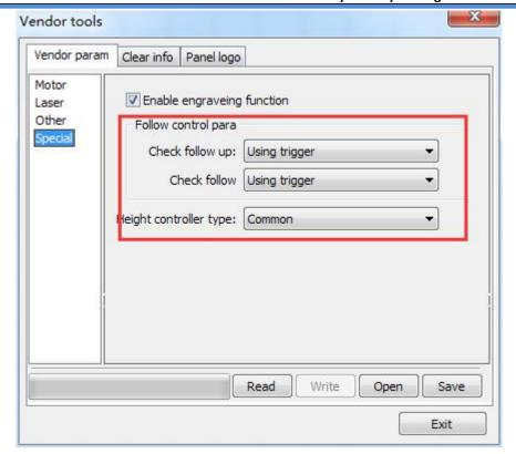
User still can selet the "check follow up" to be "use delay" and the "check follow" to be "using trigger".
