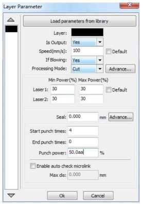
For laser piercing, the motion controller support CW piercing and pulse piercing mode. To set the piercing mode in the user parameters and layer parameters.
