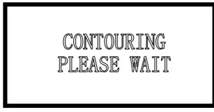
When contouring finished, system will return to main interface. When contouring, only **START** and **STOP** can be used.
