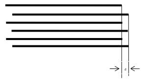
There is Backlash Compensation set in the Engrave Set of the Machine CFG. The backlash can be negative or positive value. Change the engrave step to 2mm, backlash 1mm, and start processing. If d increase, change it to a negative value; if d decreases, increase the number. Gradually d will near 0 after several adjustments. The value of the Backlash Compensation differs from different speed; you should set it according to different speed range.
