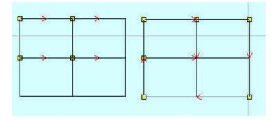
The left side is made up of 4 rectangles and the right side is processed. There are only 6 lines. This is very useful for array copy rectangles to improve the processing efficiency.
