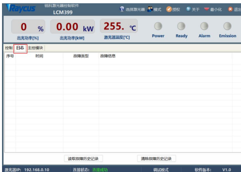
Figure 12 The alarm interface
