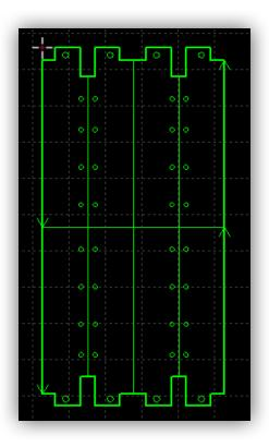
The geometries merged common lines will be integrated as a group. If the part design has in-part geometries, group the shapes within this part then make common line, otherwise software cannot identify geometry relations and sequence.
