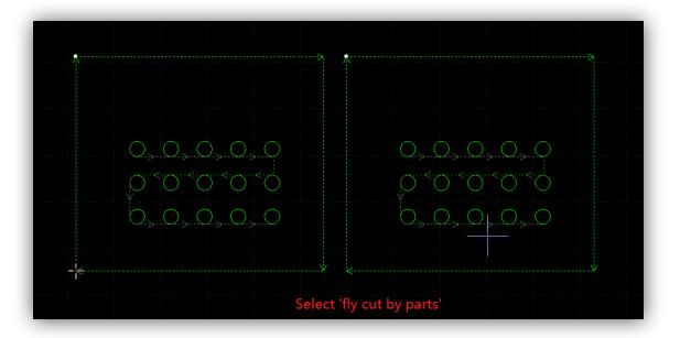
There is a parameter 'FlyCut overcut' in 'Global Parameter' window to add extra cutting at the end of each part to make sure parts are fully cut off.
