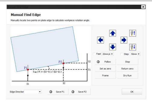
Choose one side of plate, then locate laser head to P1 and P2 position save the setting, software will calculate the plate placement angle and offset into coordinate automatically.
