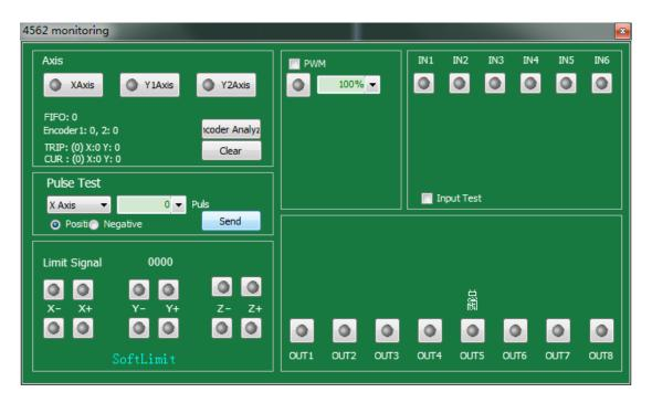
In left zone displays each motor axis number and pulse feedback from encoder. User can send given pulse commands to single axis motor check if pulse equivalent set right. Limit monitors if laser hits the limit sensor. PWM monitors laser status of
