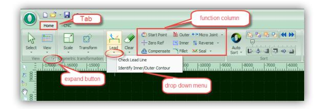
There are two tabs of Home and CNC, click each tab open the sub-menu. There will be a third tab 'Working' when machine in a cutting process.
