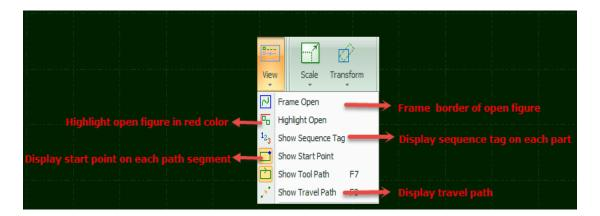
Click the option you can see feature tags applied on drawing immediately. The option button in yellow indicates the option activated. If the option button not in yellow color means function not enabled. For example, is enabled, graphic will show the tool path with arrow symbol, close the arrow symbol disappear.
