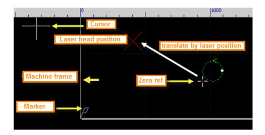
If the red cross mark does not match the real position of laser head, please check the mechanic origin and correct the origin by CNC > Return Origin. If click Preview on control panel, the drawing crossed white box on screen, it indicates the cutting zone will exceed machine bed.
