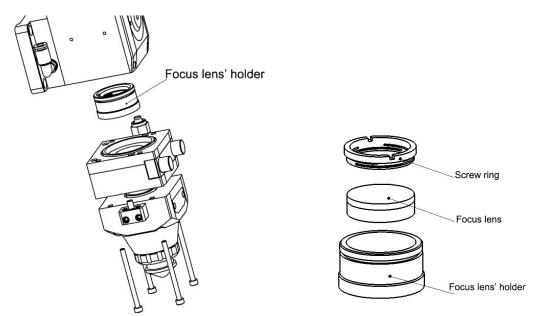
Figure 14. Focus lens with lens' holder.
