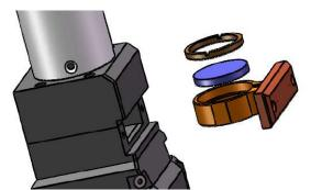
Figure 11. Protective windows of collimate lens.
