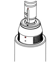
Figure 7. The insertion and locking of QBH fiber.
