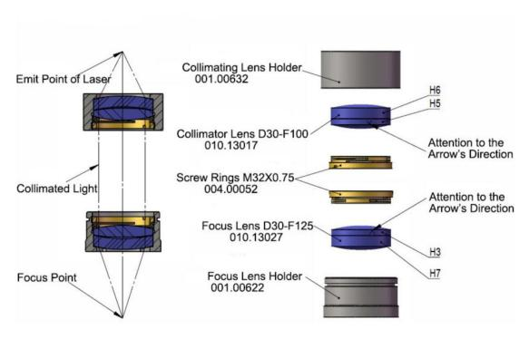
Figure 16. Collimate and focus lens' assembly process of A200M Cutting head.
