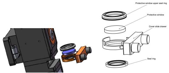
Figure 12. Protective windows of focus lens.
