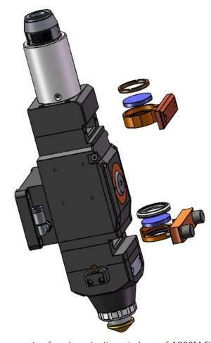
Figure 10. The components of each protective windows of A200M fiber laser cutting head.
