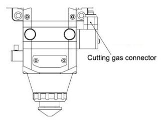
Figure 5. The interface of cutting gas of A200M fiber laser cutting head.
