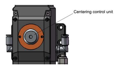
Figure 9. Focus adjustment unit of A200M fiber laser cutting head.
