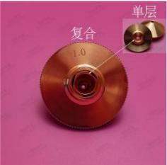
A double nozzle with a conical inner wall and a central hole, shown against a pink background. A small inset shows a single nozzle labeled '单层' (Single) and the main nozzle is labeled '复合' (Composite). | 双层复合在单层的基础上加了内芯      | 双层 2.0 大小以上用于碳钢砂面切割 |
