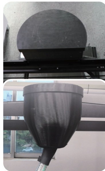
3 Fill with material and cover with barrel cover. 料装满后盖上漏斗盖。
