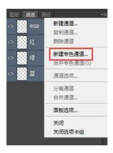
3. Establish a new special color channel (color and density data will not affect the actual printing white ink thickness)
