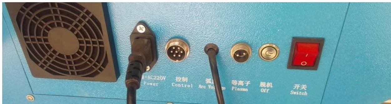
**WARNING: Arc voltage is polarity sensitive and care should be taken not to connect in reverse. Best case scenario the arc insurance fuse will blow, worst case scenario one of the components on the PCBs will blow leading to costly replacement. If unsure of connection please whatsapp 0606006000 for further guidance.**
