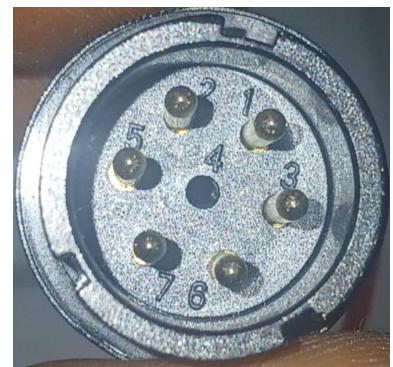
On this new connector Pin 1 and 2 are used for the plasma signal. Connections are not polarity sensitive hence can be connected anyhow to the PLASMA connection on the
