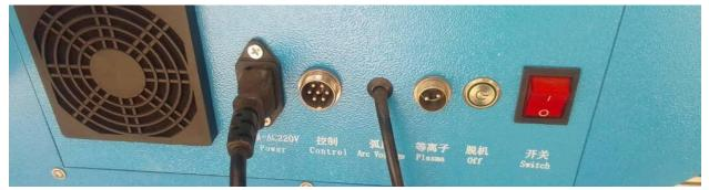
WARNING: Arc voltage is polarity sensitive and care should be taken not to connect in reverse. Best case scenario the arc insurance fuse will blow, worst case scenario one of the components on the PCBs will blow leading to costly replacement. If unsure of connection please whatsapp 0606006000 for further guidance.
