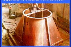
Using Tradesman in a Box™, this square to round transition was completed quickly and accurately first time. The development even included the line marking and number of degrees for forming every bend!
