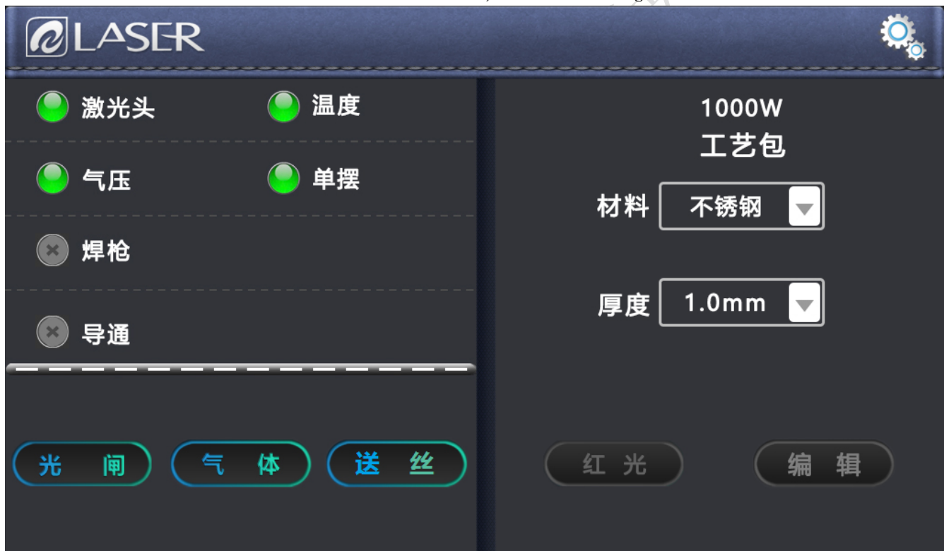
Main interface, schematic diagram
