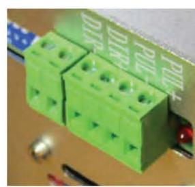
New 2022+ Model Rotary Connector Changed to 5 cords, so it able to provide 24V output for rotary if needed
