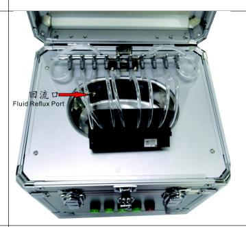
Step8 往清洗槽中倒入清洗液,一直到液面接近回流口。 Pour cleaning fluid into the cleaning tank ,to close to the water outlet port
