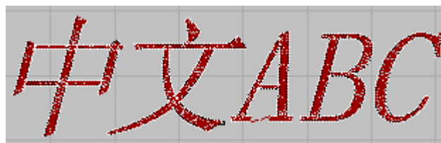
The effect of stitch whose tilt angle is set at 15 degrees
