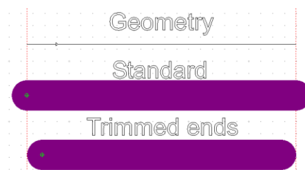
. Visualization of the same path without or with Trimmed ends enabled
