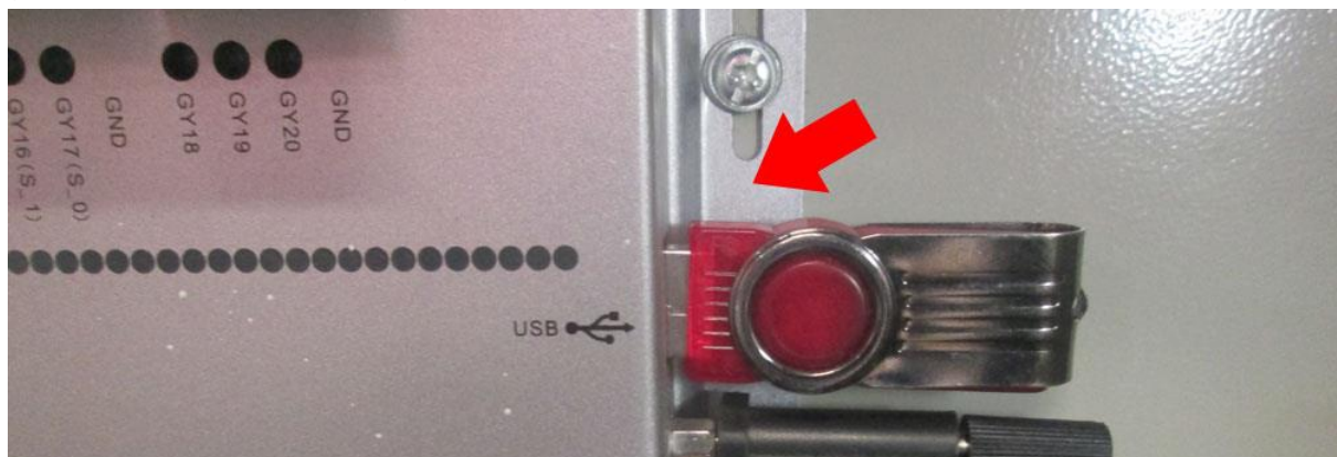
Plug in the Flash Drive Directly onto the EasyRoute DSP Control System (Motherboard). This is to avoid any communication interference or error during backup/restore process.
