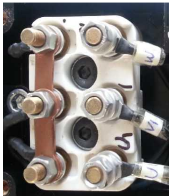
380 V star connection method
