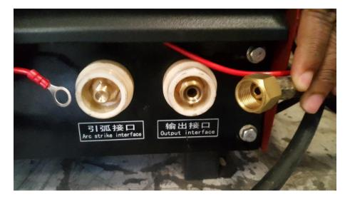
Please note that if the red wire is not connected you still will be able to cut, but only arcing when the torch touches the plate to create a circuit.
