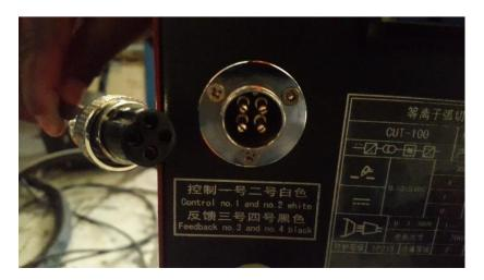
Connect the Red connector cable to the Arc Strike Interface and the Nut Connector to the Output Interface.
