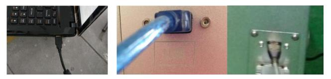
USB line, connect the control cabinet and computer, as in the above pictures.
