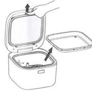
1. Toggle the latch to eject the press frame.
